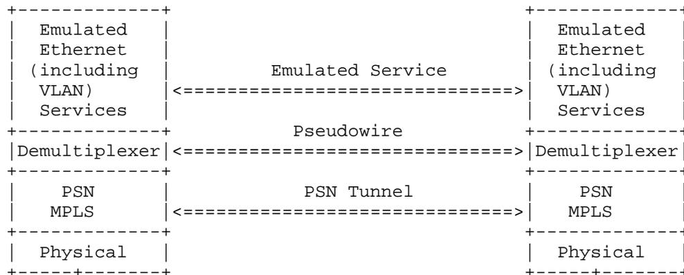
Figure 2: Ethernet PWE3 Protocol Stack Reference Model
